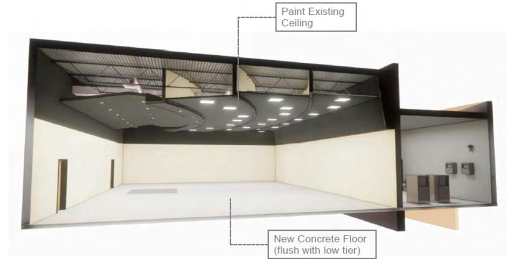
Tiers Demolished and New Concrete Flat Floor
